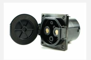
The SKZ series GB/T DC charging socket is installed on the electric vehicle and realizes the DC charging function by cooperating with the DC charging cable. The product meets the requirements of GB/T 20234.3-2015 and RoHS.
